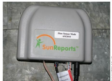
A SunReports sensor box collects data and sends it out to a web portal for remote monitoring of temperatures and pump status from anywhere with internet access.
